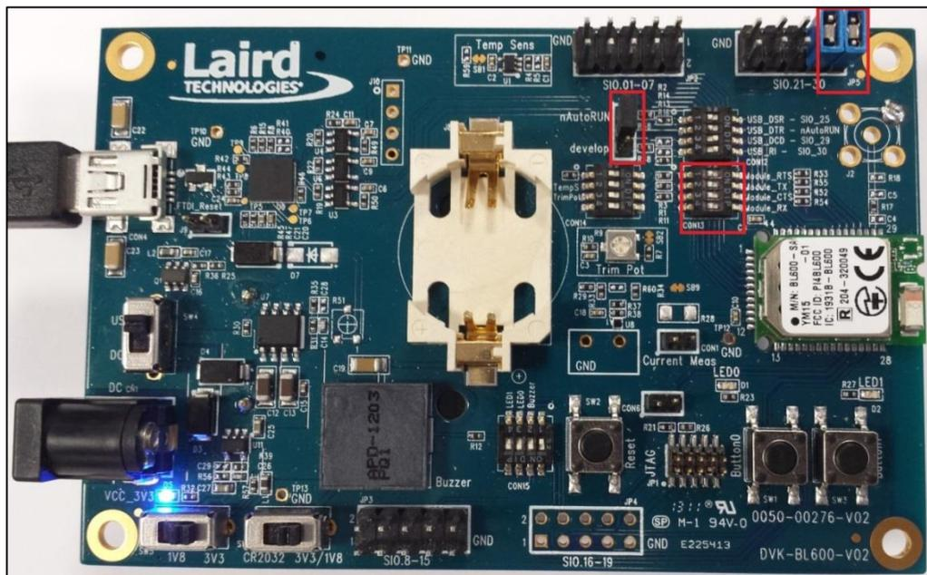
Figure 11: Host less autorun configuration
