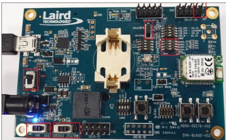
*Figure 2: Switch and jumpers position*
